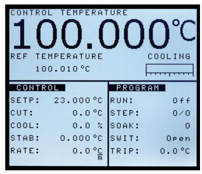
Metrology Well displays offer all the information deeded to perform calibrations—control and reference probe temperatures, heating and cooling status, set-point temperature, stability criteria, and more.
