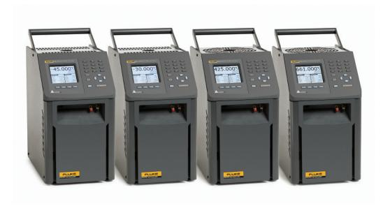
The Metrology Well family consist of four models (Model 9170, 9171, 9172, amd 9173) which, combined, cover a temperature range of -45  $^{\circ}$ C to 700  $^{\circ}$ C.
