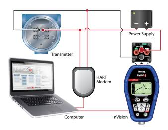
nVision Reference Recorder connections
