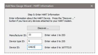
The *Manufacturer ID*, the *Device type ID* and the *Device ID* combined together form the unique ID, defined by the manufacturer, that is used to communicate with a smart transmitter during the calibration session. This ID can be entered manually by consulting the transmitter documentation or determined automatically by FastCalXP.
