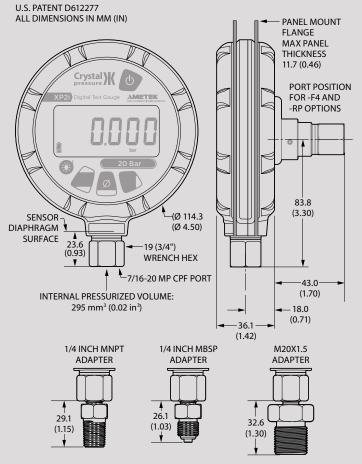
ADDITIONAL SENSOR LENGTH WITH OPTIONAL FITTING ADAPTERS
