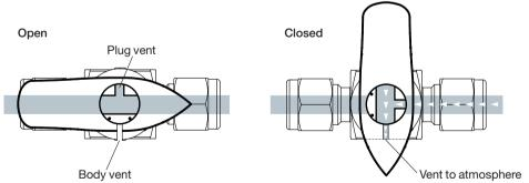
• In close position the plug valve allows to release the pressure to the atmosphere
