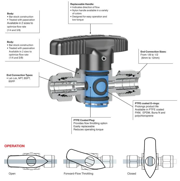
• Valve is capable of bi-directional flow (please note maximum differential pressure is limited to 150 psig when flow is reversed)
